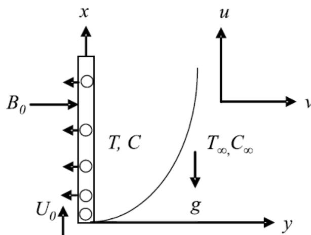
Fig.I. Flow configuration and coordinate system
